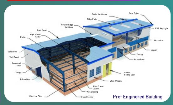
Pre engineered building is a steel structure built over a structural concept of primary members, secondary members, and the cover sheeting connected to each other. The structural members are custom designed to be lighter in weight as well as high in strength.
